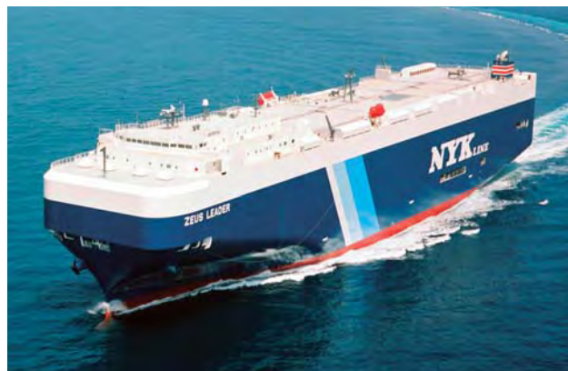
ZEUS LEADER a 18,697 dwt vehicles carrier built by Mitsubishi Heavy Industries, Ltd. Nagasaki Shipyard & Machinery Works for Nippon Yusen Kabushiki Kaisha.
