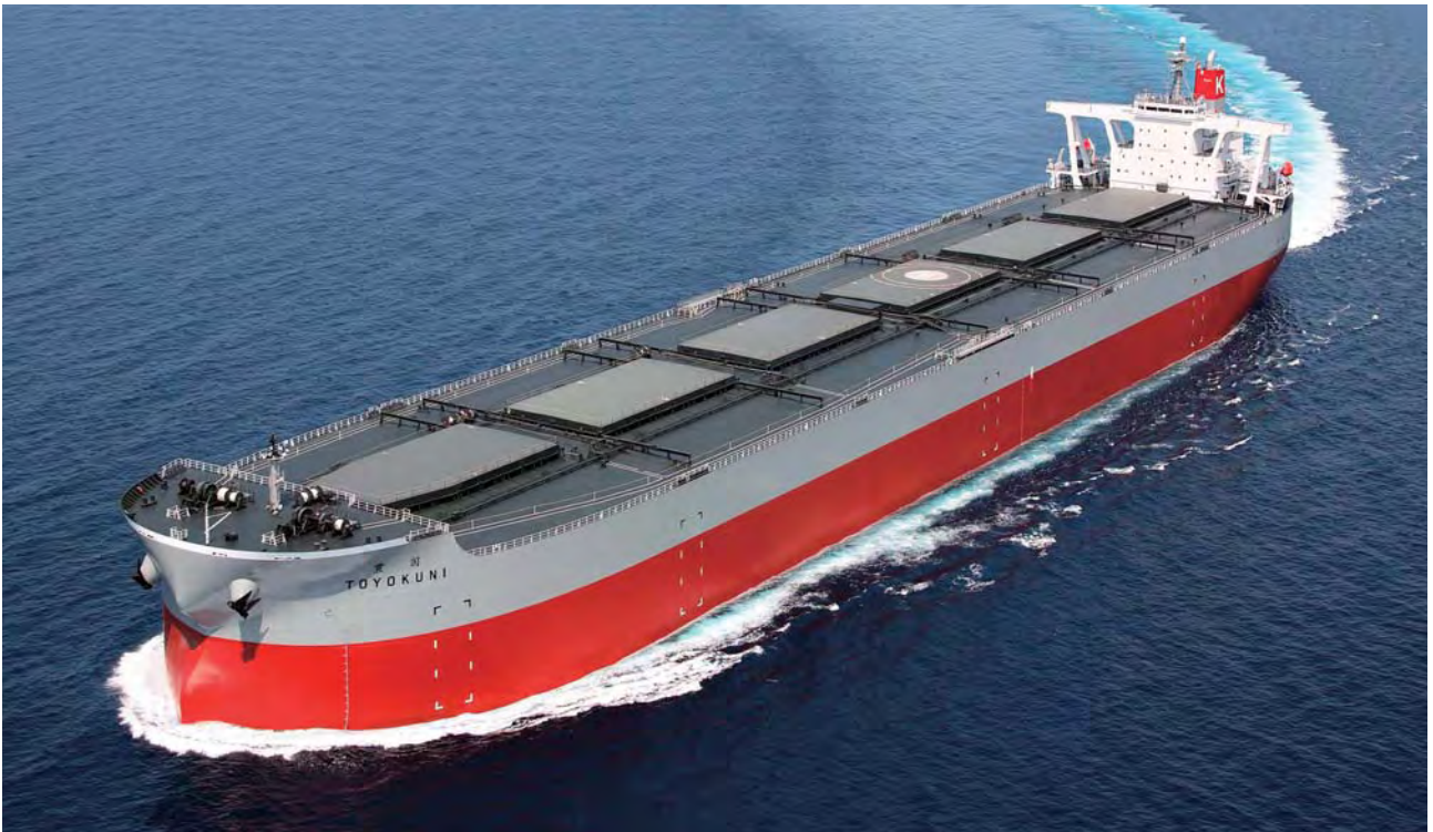
TOYOKUNI a 297,584 dwt ore carrier built by Universal Shipbuilding Corporation, Ariake Shipyard for Kawasaki Kisen Kaisha, Ltd.
