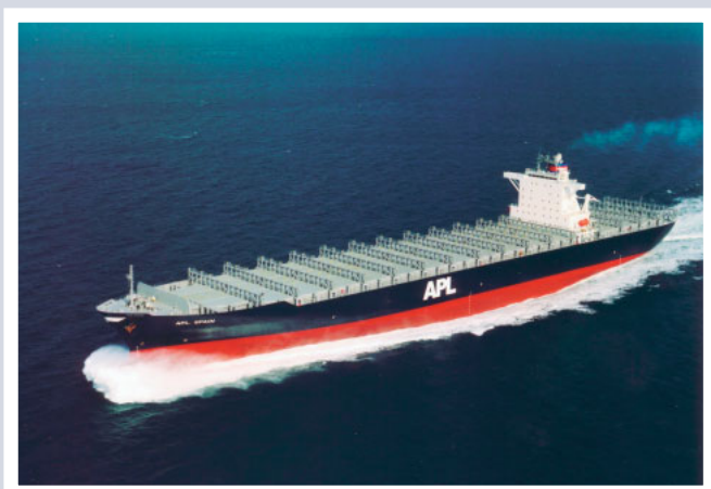
APL SPAIN A 67,009 dwt container carrier built by Koyo Dockyard Co., Ltd., for Southern Route Maritime S.A.
