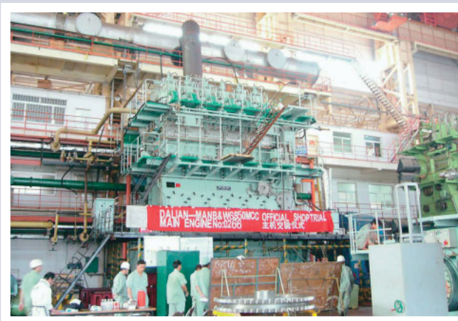
A shop trial for a main engine at Dalian Marine Diesel Works
