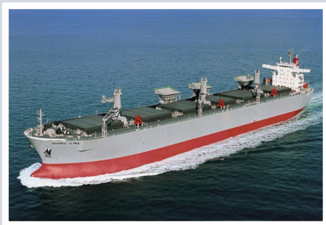
UNIVERSAL GLORIA A 62,716 dwt chip carrier built by Imabari Shipbuilding Co., Ltd., for Manatee Navigation S.A.
