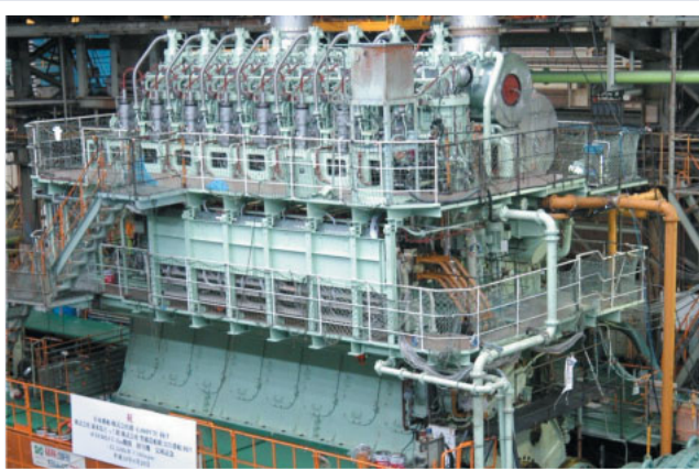
The first electronically controlled marine diesel engine, known as the UEC Eco-engine, developed at Mitsubishi Heavy Industries, Ltd., Kobe Shipyard & Machinery Works
