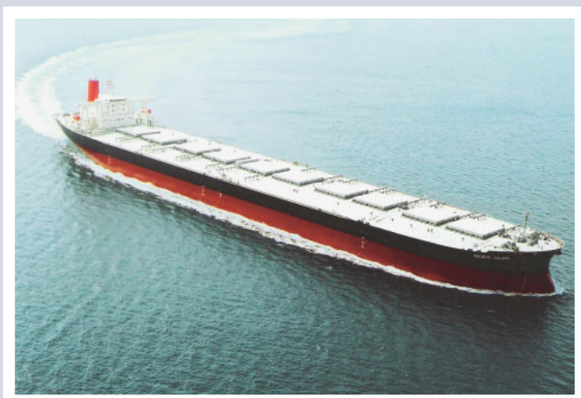
PACIFIC GLORY A 233,694 dwt ore carrier built by Imabari Shipbuilding Co., Ltd., for Fir Shipping S.A.
