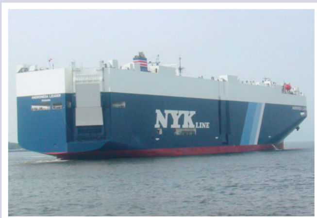
ANDROMEDA LEADER A 21,443 dwt vehicle carrier built by Toyohashi Shipbuilding Co., Ltd., for ANZ National Bank Limited.
