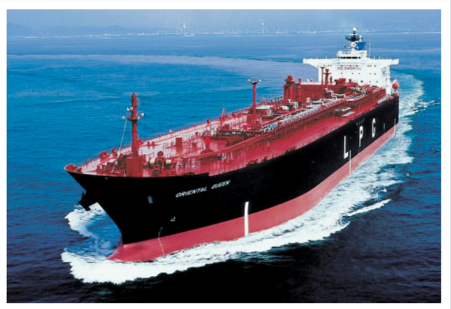
ORIENTAL QUEEN A 82,000m 3 LPG Carrier built by Universal Shipbuilding Corporation for Phoenix Navigation Corporation Limited
