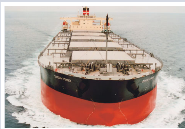
GREEN POWER A 89,999 L/T dwt bulk carrier built by Oshima Shipbuilding Co., Ltd., for Laurel Maritime Co.Ltd.
