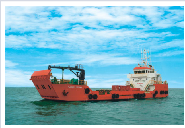
AJANG MEDINA A 430 dwt oil spill recovery vessel built by Shin Yang Shipyard Sdn. Bhd. for Ajang Shipping Sdn. Bhd.
