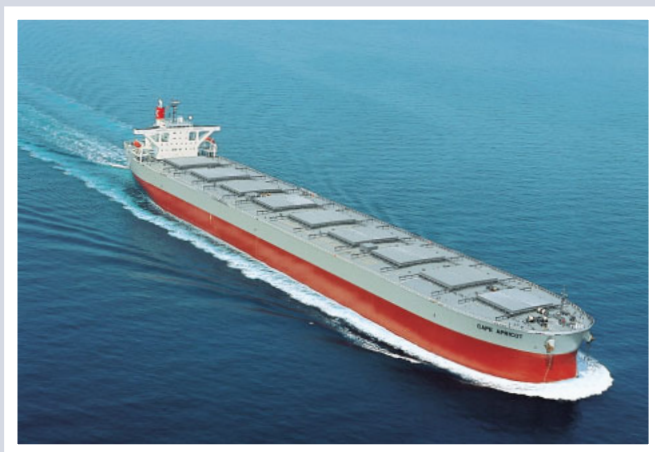
CAPE APRICOT A 180,310 dwt bulk carrier built by Koyo Dockyard Co., Ltd., for Leo Ocean, S.A.
