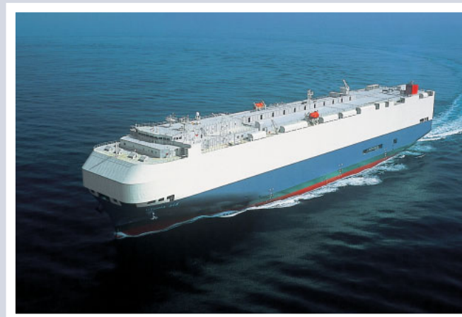
UTOPIA ACE A 19,086 dwt vehicle carrier built by Mitsubishi Heavy Industries, Ltd., for Orchard Maritime (Panama) S.A. (This design was awarded Ship of the Year at the Lloyd's List Maritime Asia Awards)
