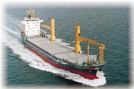
Ratha Bhum —the 6,393 gt container carrier built by Kyokuyo Shipyard for Regional Container Lines
