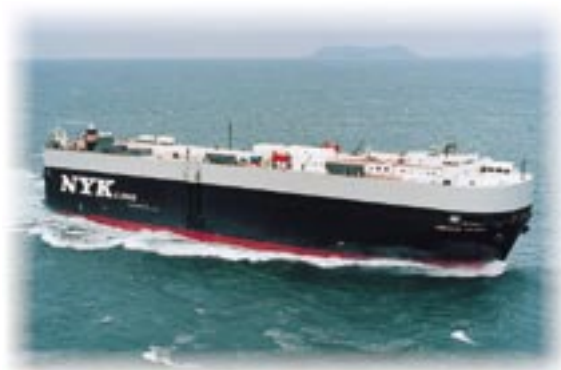
Hercules Leader —a 57,449 gt vehicle carrier built by Imabari Shipbuilding for Hong Kong-based managers
