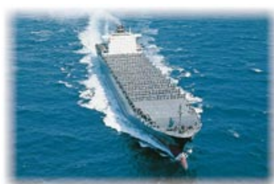
NYK Sirius—a 76,847 gt container carrier constructed by Mitsui Engineering & Shipbuilding for Columbia Shipmanagement
