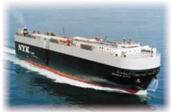
Delphinus Leader —a 57,391 gt vehicle carrier built by Imabari Shipbuilding for Milford Shipholding S.A.
