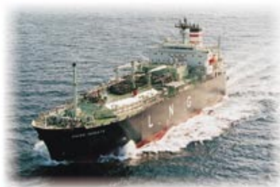
Aman Hakata —an 18,942 m 3 LNG tanker constructed by NKK Corporation for Asia LNG Transport Dua (Malaysia)
