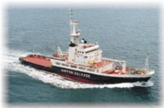
Koyo Maru —a 2,096 gt ocean-going salvage tug built for Japan Ocean Tug and Nippon Salvage by Mitsubishi Heavy Industries
