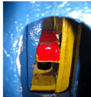
Securing device in place Hydraulic operated wedge
