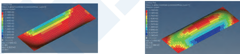
(a) Compression side (b) Tension side Figure 13 Von Mises stress at ultimate strength
