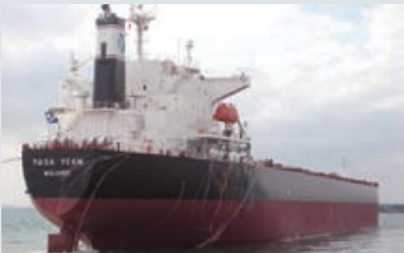
YASA TEAM Sanoyas Hishino Meisho公司为YA-SA Shipmanagement and Trading S.A.公司承建的75,621 dwt散货船
