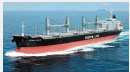
DAIWAN BRAVE 21,514 gt BULK/LUMBER CARRIER built by NAMURA SHIPBUILDING CO., LTD. IMARI SHIPYARD & WORKS for KATAGALAN STAR S.A
